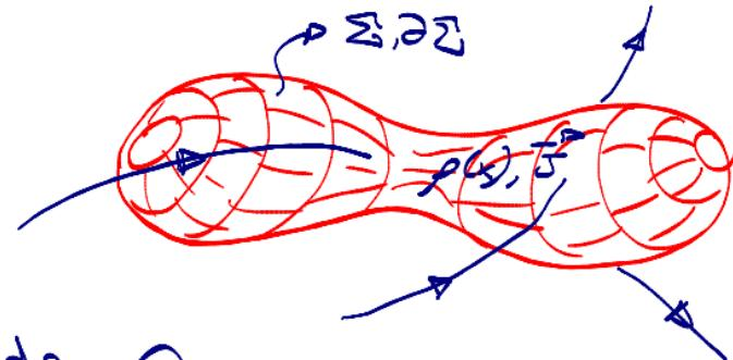
$$\oint_{\Sigma} \frac{\partial u}{\partial t} d\sigma + \oint_{\Sigma} \vec{f} \cdot \vec{\vartheta} d\sigma + \oint_{\Sigma} \vec{\nabla} \cdot \vec{s} d\sigma = 0$$
